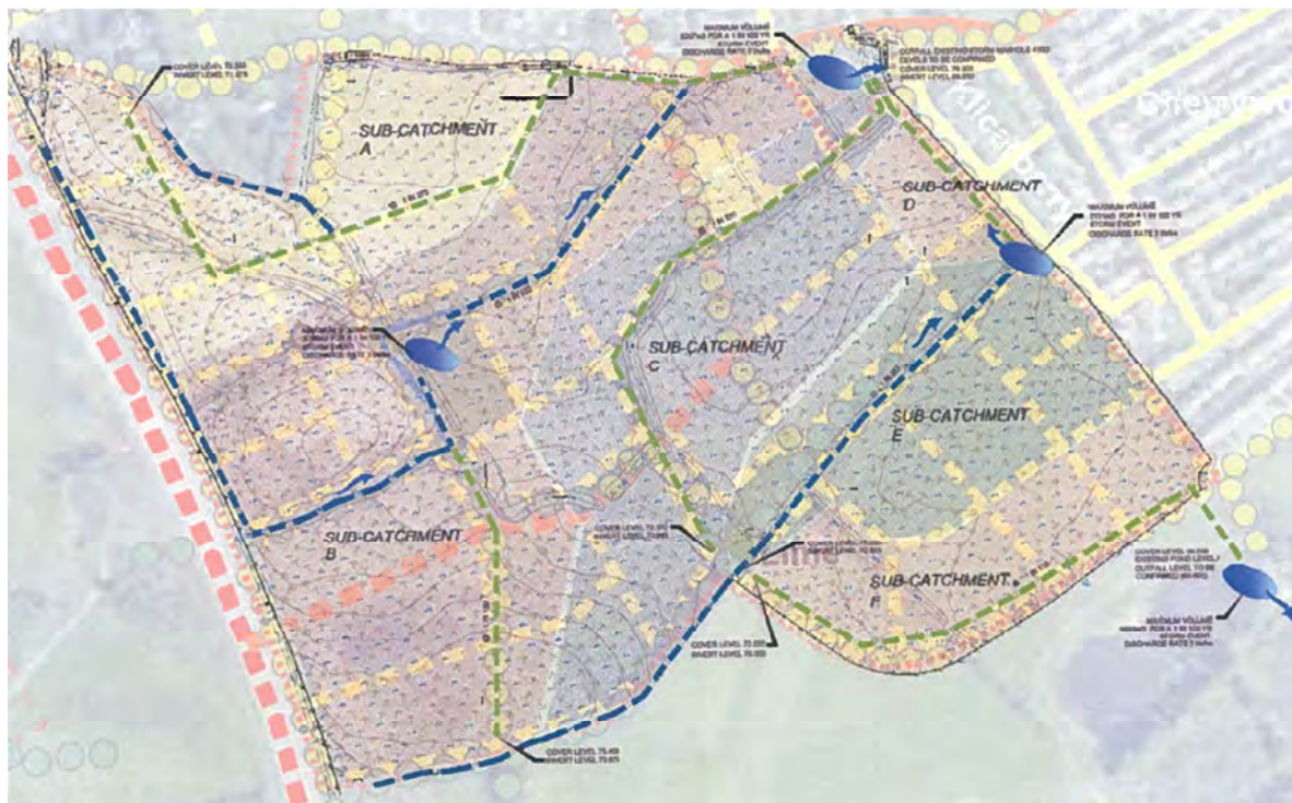
Figure 4.4 Proposed surface water drainage layout
